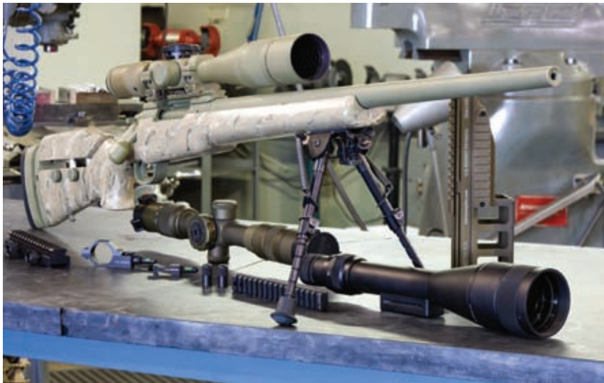
One of the company's test rifles, a duplicate of the current USMC-issue sniper rifle. Note the mount here and below. U.S. Optics manufactures its own line of mounts and hardware.
